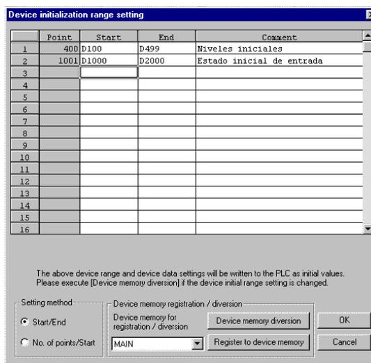
The 'Device initialization range setting' dialog box shows a table for defining initial values for device memory points.
