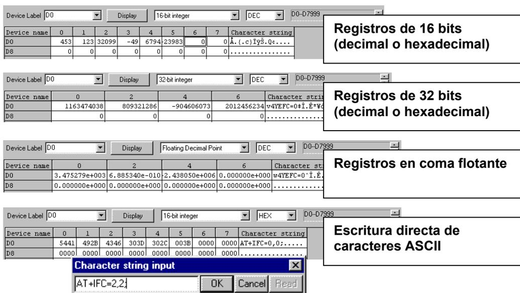
The screenshots show the 'Device memory' configuration window in GX Developer. Each screenshot shows a table of device addresses (D0-D8) and their values, with a callout box explaining the format.
